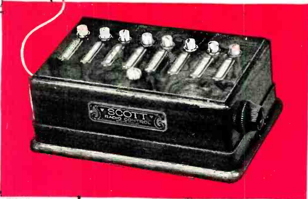
By simply pushing buttons, the desired stations are switched in or out. The knob at the end is for volume control.
