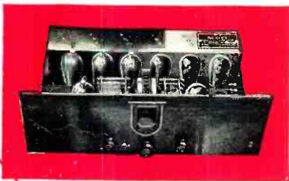
The chassis of the Scott A-C Shield Grid is a jewel of engineering precision. Four screen grid tubes are used. The overall amplification obtained is far greater than that obtained in any other receiver we know of.
